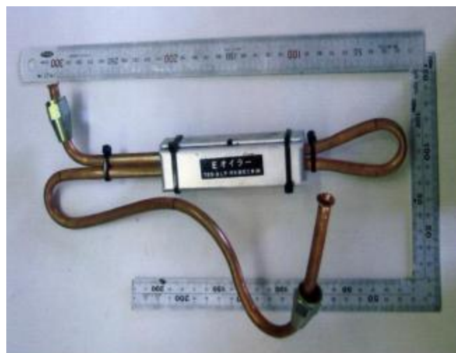
The upper photograph is copper tube assembly for a LP gas car (Nissan :Crew)
